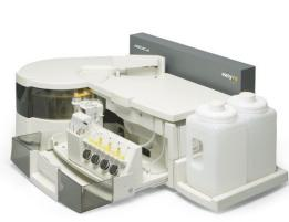
The unique slide-out drawer makes maintaining the EasyRA analyzer simple by making all components easily accessible. Ion-selective electrodes and tubing are easily replaced. The "peek" position allows viewing of diluter and pumps during a sample run.
